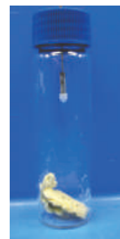
Sampling blue cheese with MonoTrap RGPS TD
