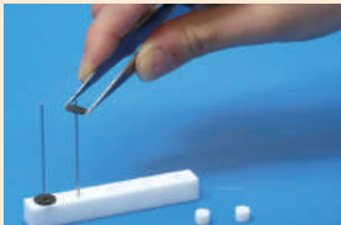
MT Holder & MT Stand Grasp the MonoTrap with tweezers and insert the holder into the hole on the MonoTrap.
