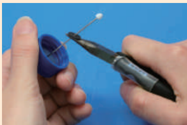
Hold MT Holder with pliers whose ends have been cleaned and pass it through the septum. Put a cap on top of the holder.
