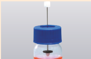
Clean Pin Hole Septum with Vial (40 mL) Tighten the septum on the vial.
